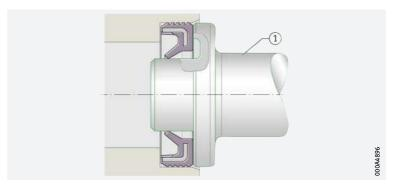
Fitting using a fitting sleeve
